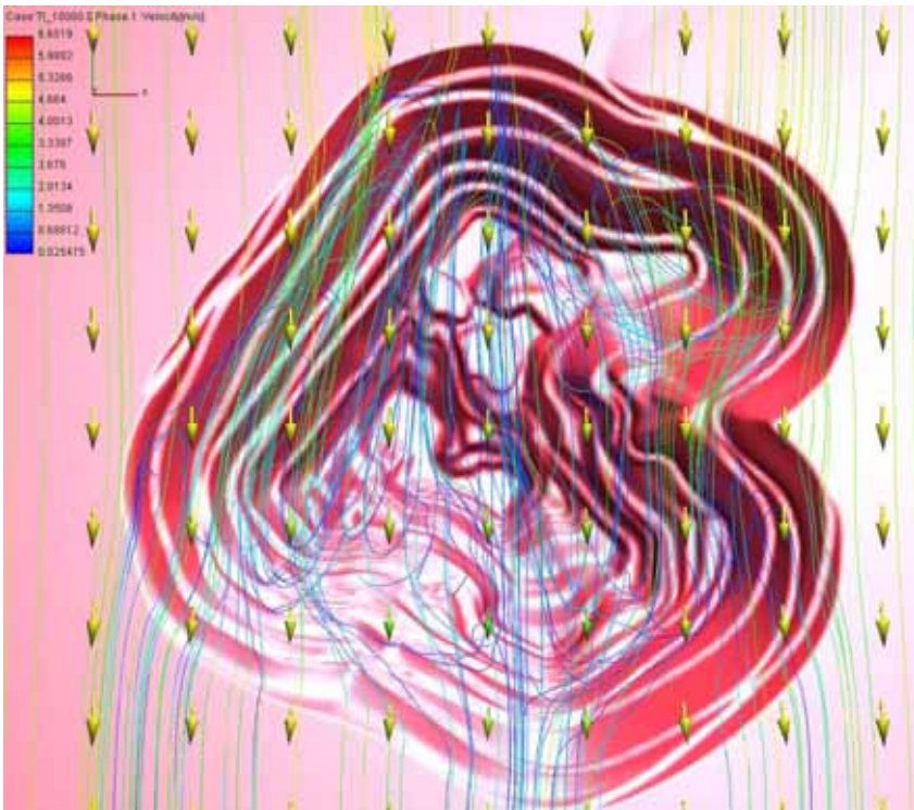
Figure 6.27: Streamlines of flow through the pit for unstable atmospheric boundary layer flow, U_{10m} = 3 \text{ m/s} .
