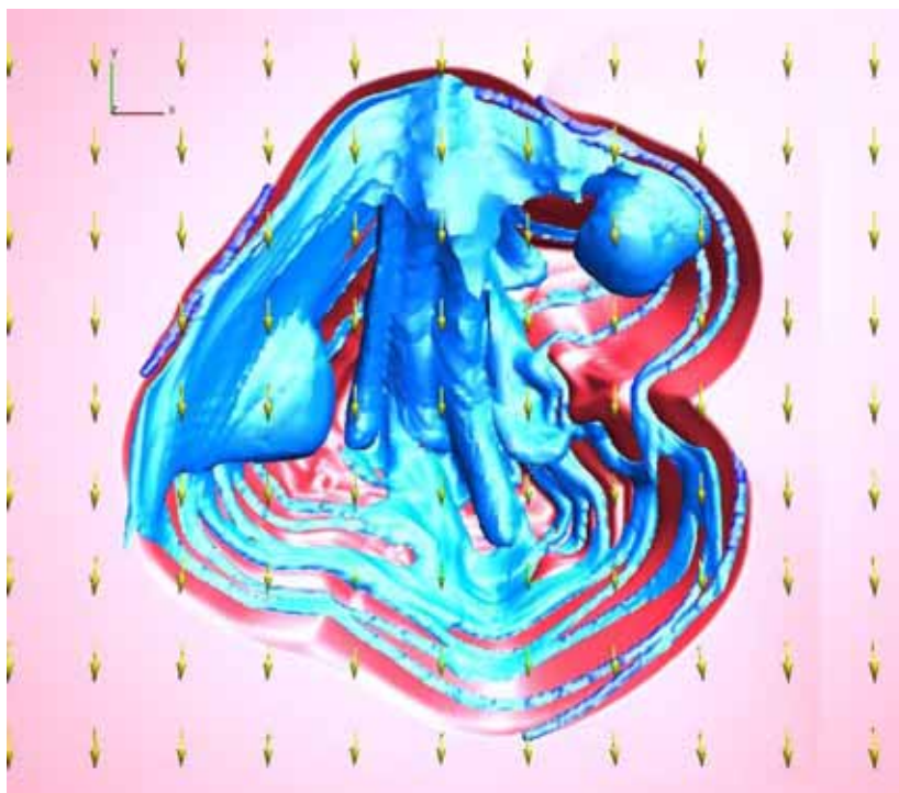
Figure 6.41: Iso-surface of Phase II volume fraction (dust concentration) ( 2e-9 ) and streamlines in the pit for unstable atmospheric boundary layer flow, U_{10m} = 3 m/s, 10 \mu\text{m} particles.
