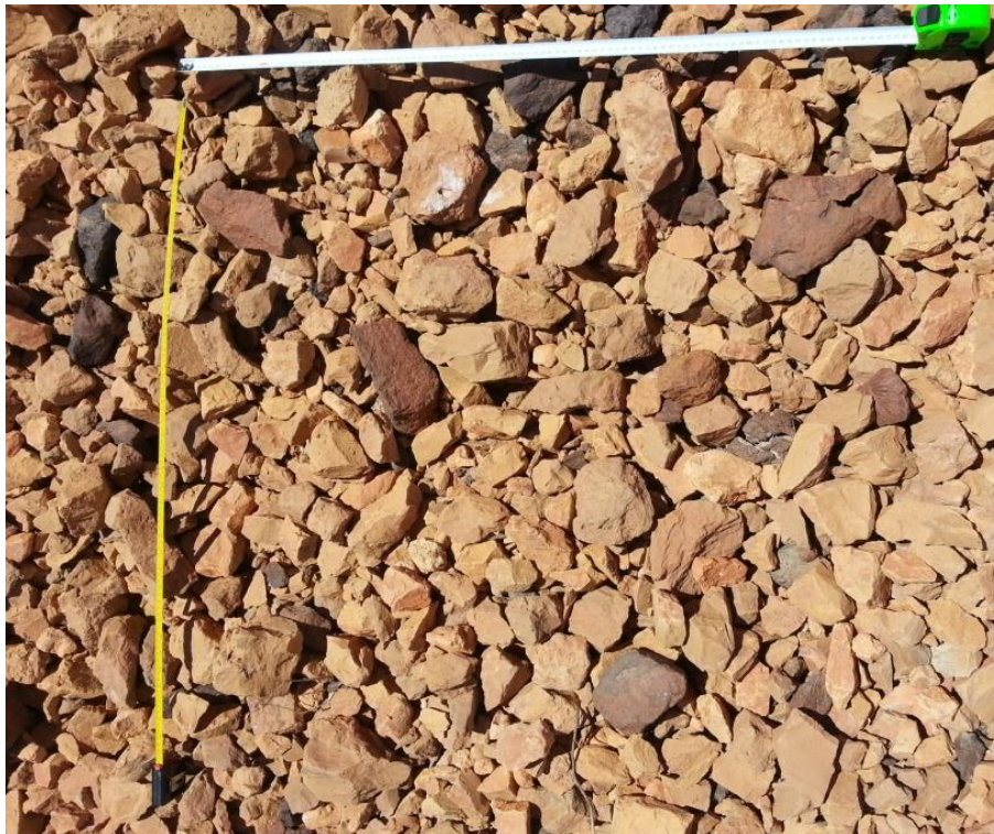
Figure 4: Cell 2 upper slope batter section with D_{50} of 43.3mm.
