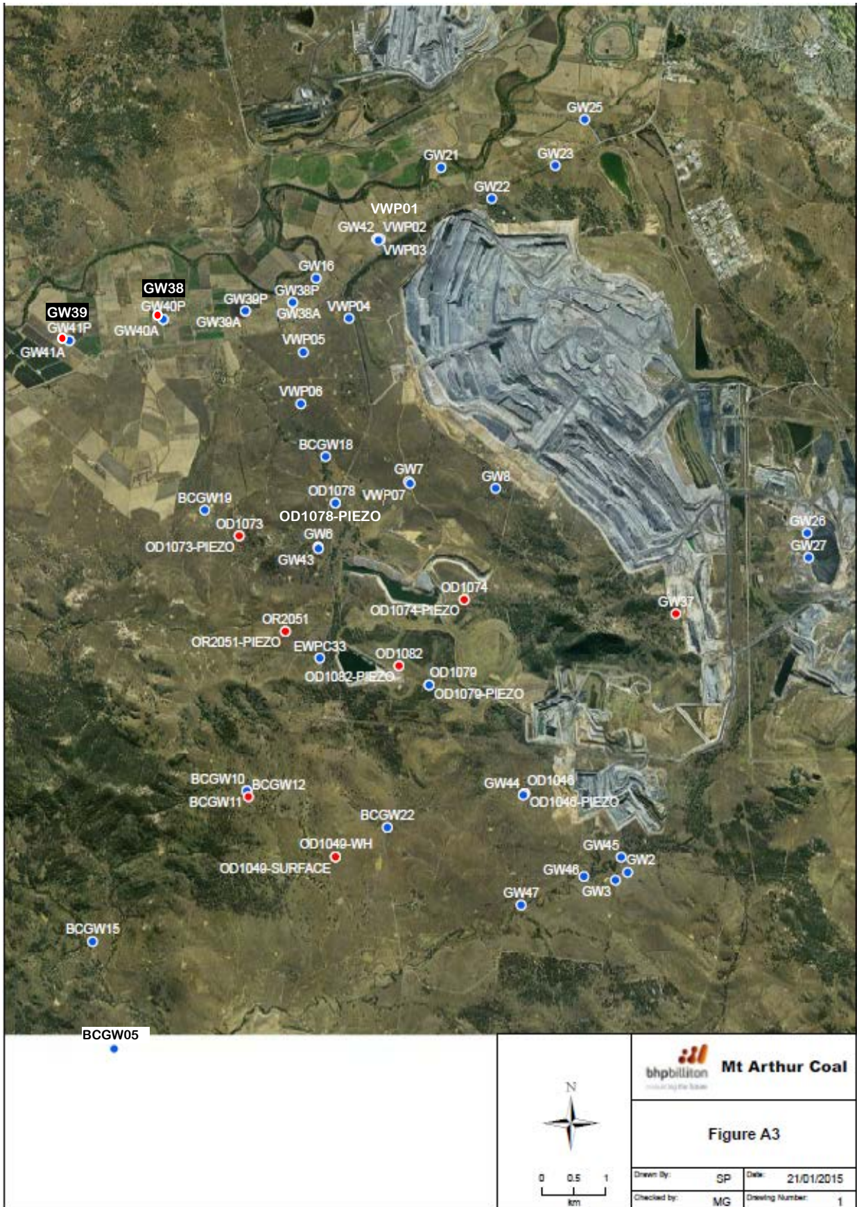
Figure A3.1: Interim Groundwater Monitoring Locations (also shows monitoring bores to be decommissioned as red points)
