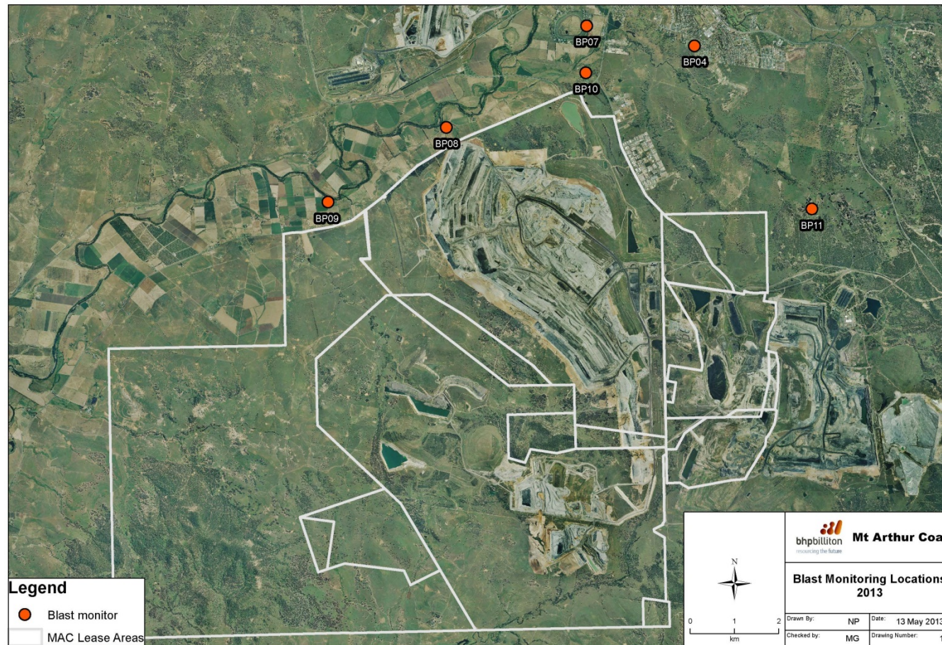
Figure 1: Blast Monitoring Location Plan
