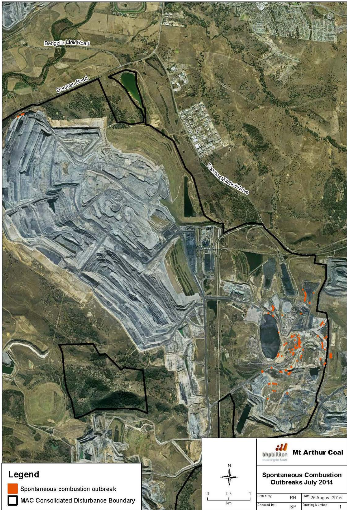
Figure 16: Locations of spontaneous combustion at Mt Arthur Coal at start of reporting period
