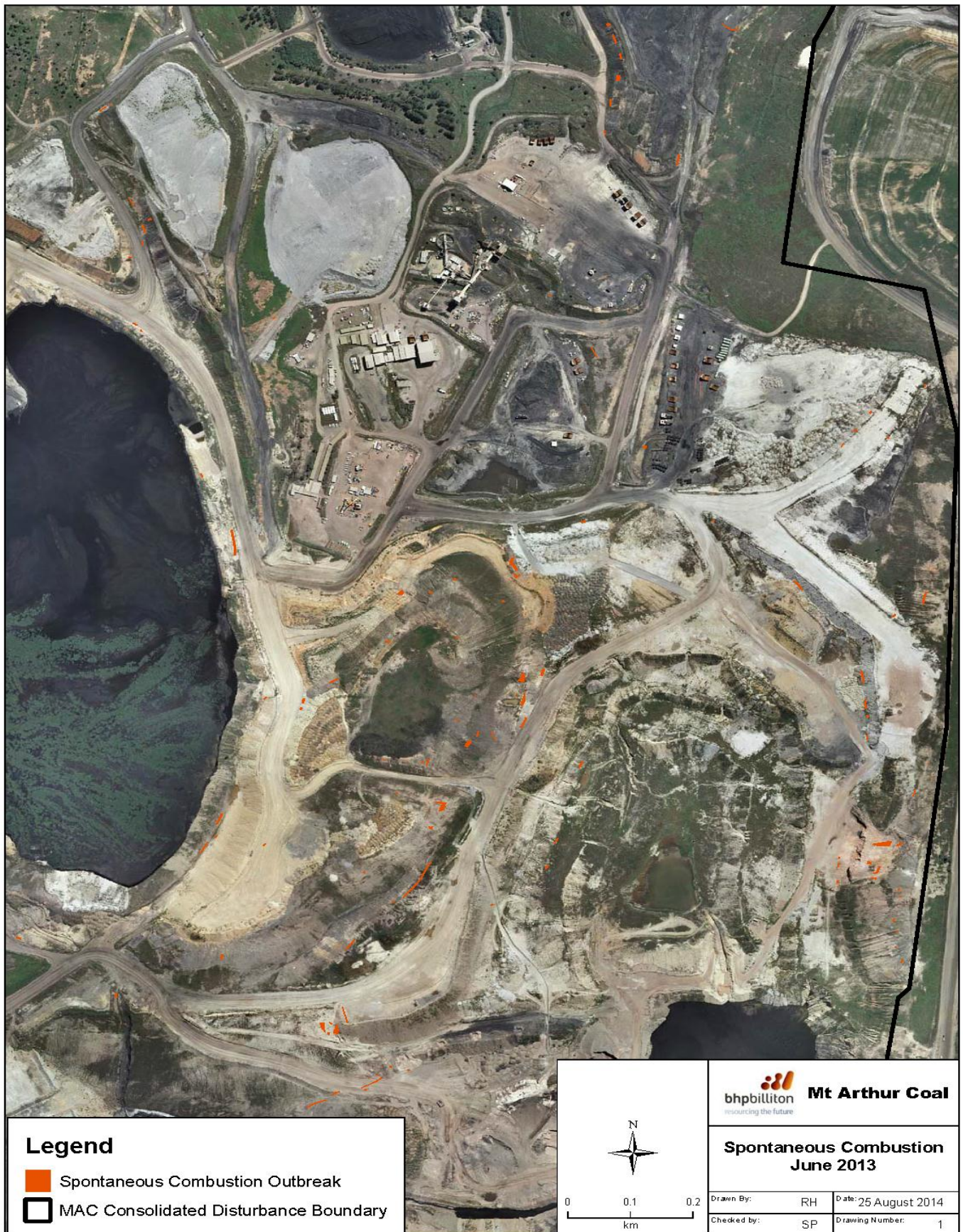
Figure 15: Locations of spontaneous combustion at Mt Arthur Coal at start of reporting period
