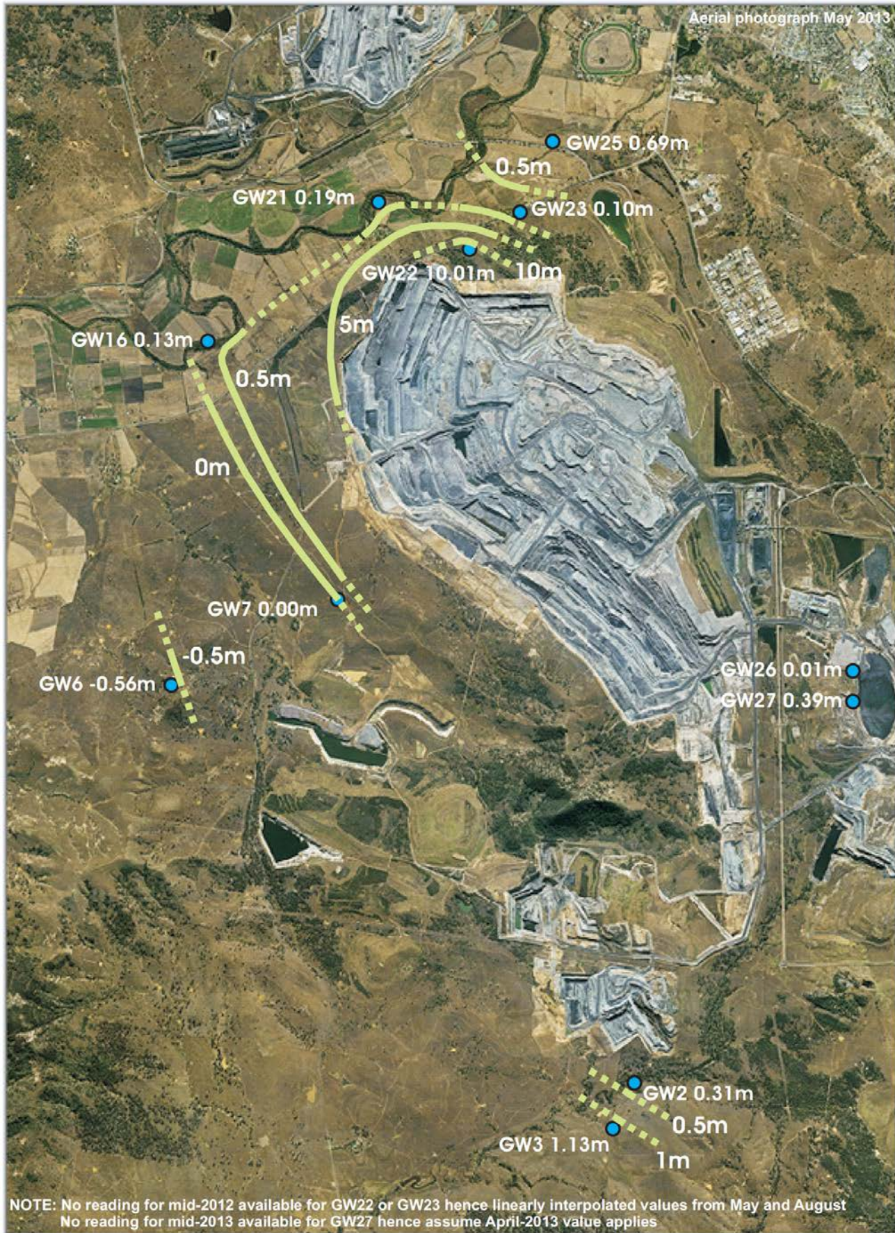
Figure 5A: Groundwater drawdown during the reporting period (prepared by Gilbert and Associates)
