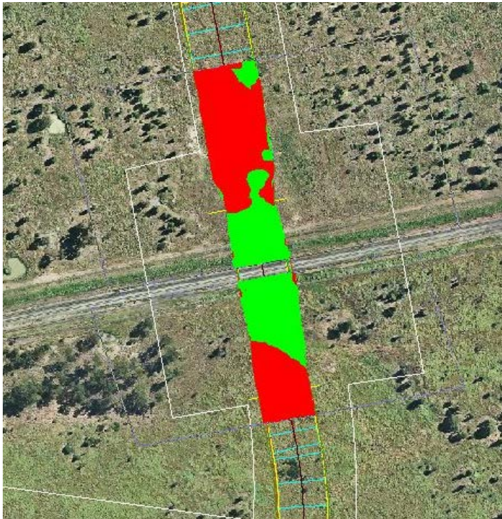
Figure 8 Crossing 3 - Goonyella Line (Rail CH130 / Alignment CH68.5) (Red: cut areas; Green: fill areas)
