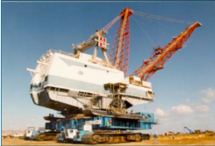
Figure 14 Dragline on tracked crawler transporter
