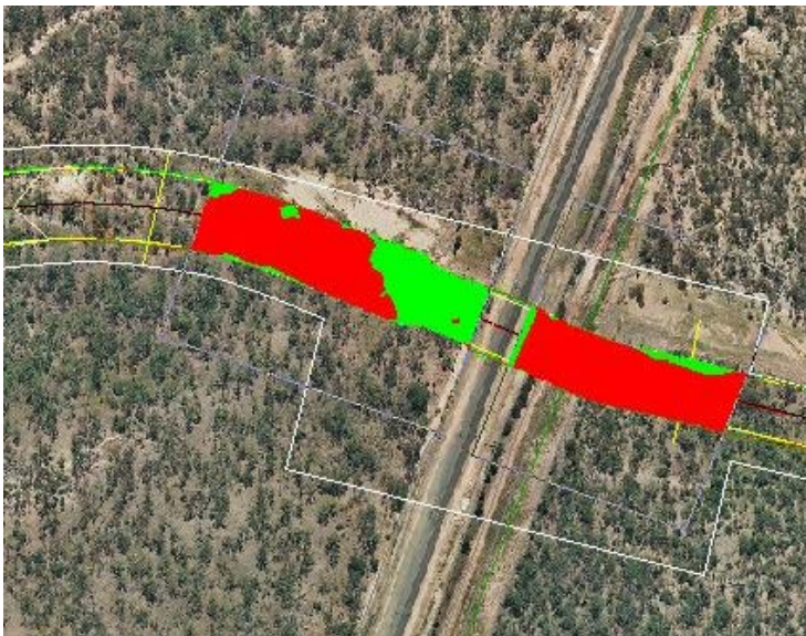
Figure 7 Crossing 2 - Norwich Park Line (Rail CH6.29 / Alignment CH47.4) (Red: cut areas; Green: fill areas)
