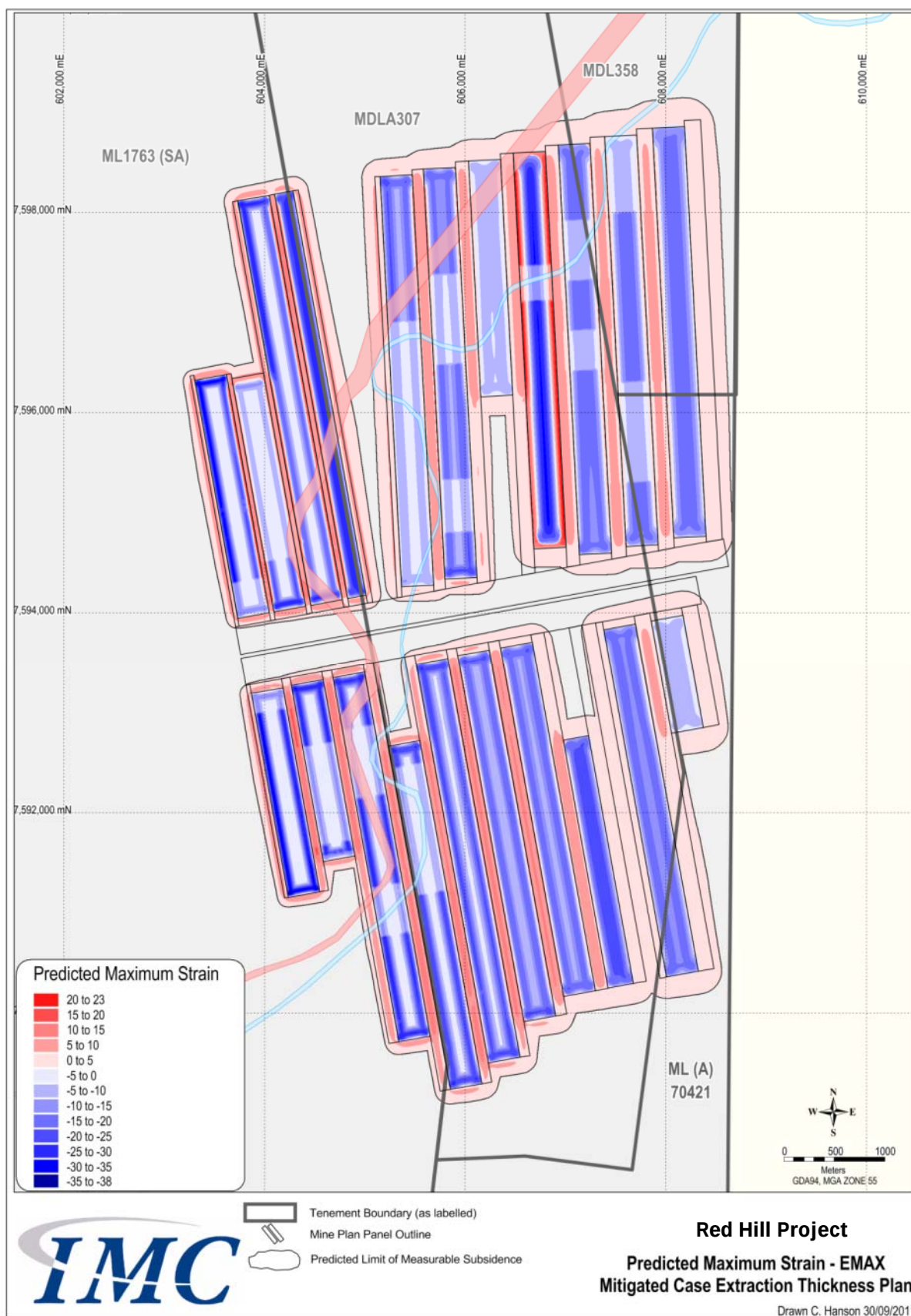
Figure 5-4 : Predicted Maximum Strain (Emax) in mm/m for RHM Mine Layout Scenario 1
