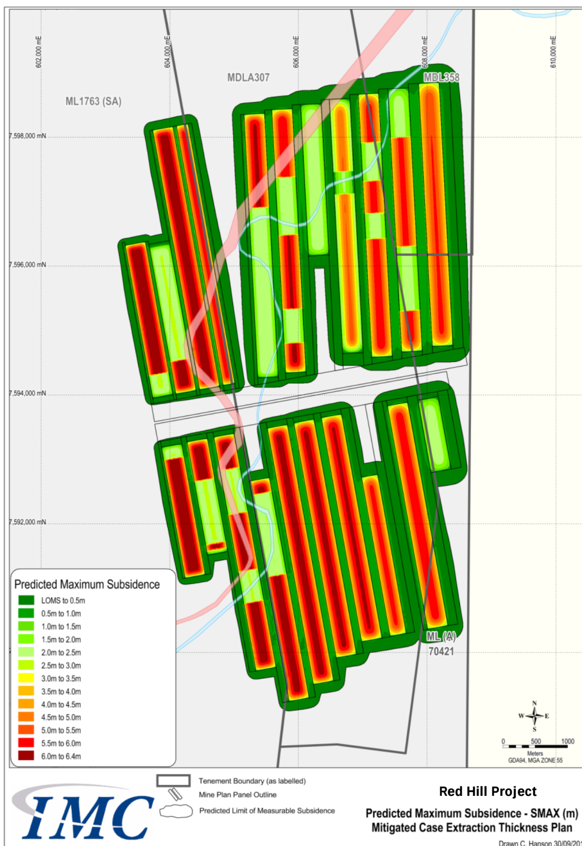
Figure 5-2 : Predicted Maximum Subsidence (Smax) in metres for RHM Mine Layout Scenario 1
