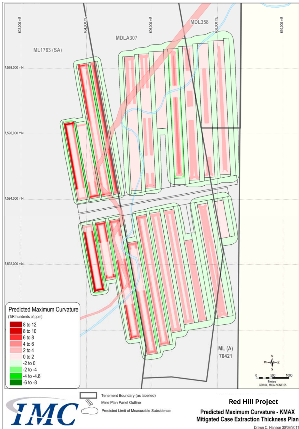
Figure 5-8 : Predicted Maximum Curvature (Kmax) in 1/R hundreds of ppm for RHM Mine Layout Scenario 1
