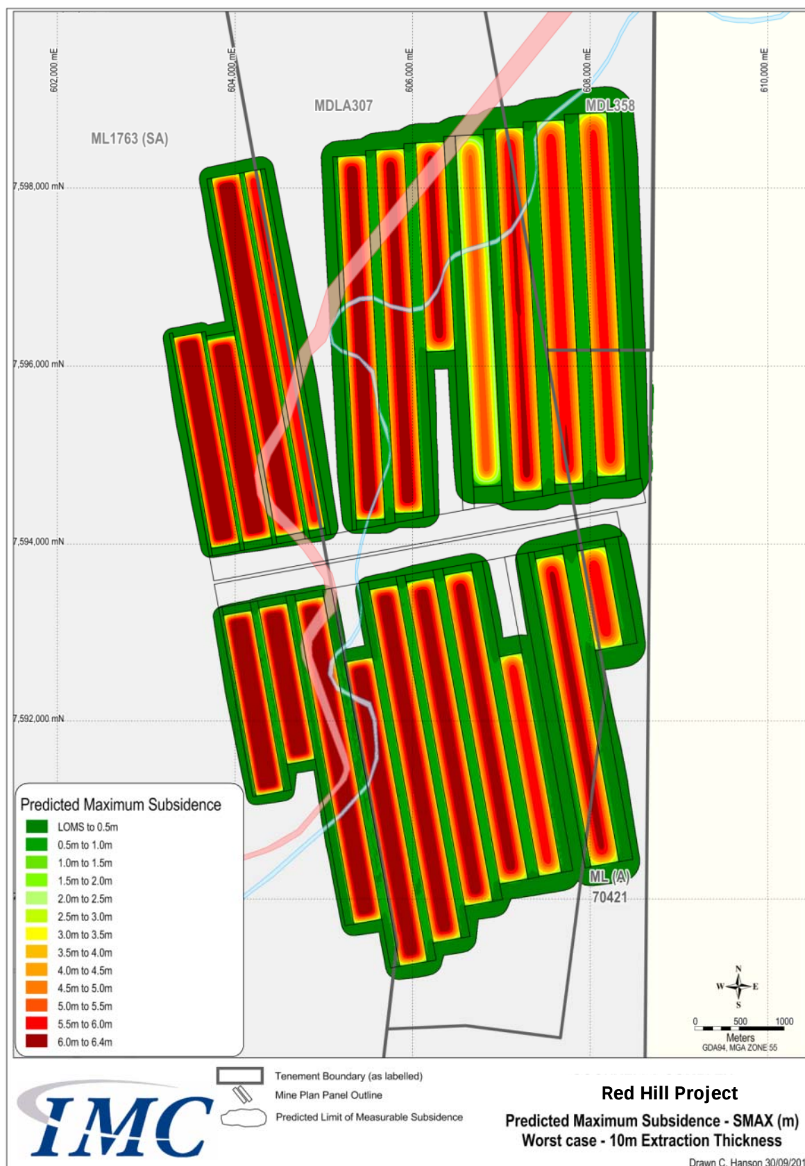
Figure 5-3 : Predicted Maximum Subsidence (Smax) in metres for RHM Mine Layout Scenario 2
