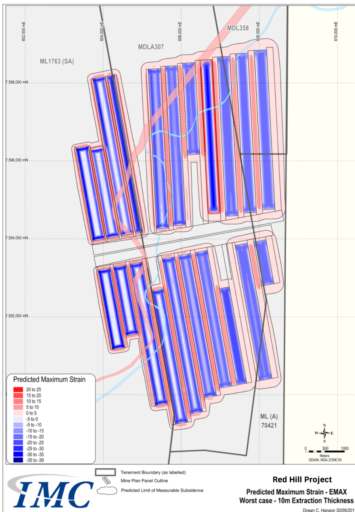
Figure 5-5 : Predicted Maximum Strain (Emax) in mm/m for RHM Mine Layout Scenario 2
