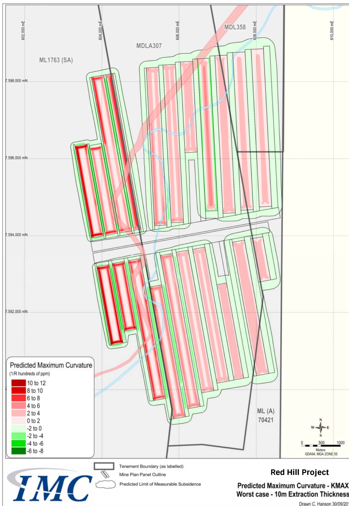
Figure 5-9 : Predicted Maximum Curvature (Kmax) in 1/R hundreds of ppm for RHM Mine Layout Scenario 2
