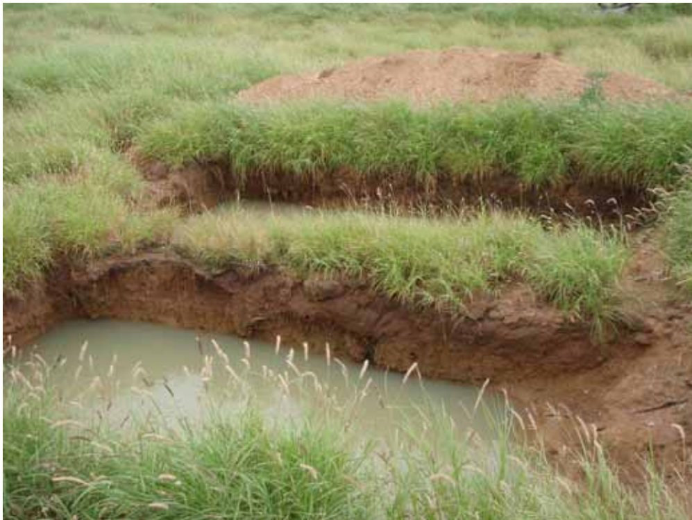
Plate 36 Drill water sumps - Peak Downs Mine
