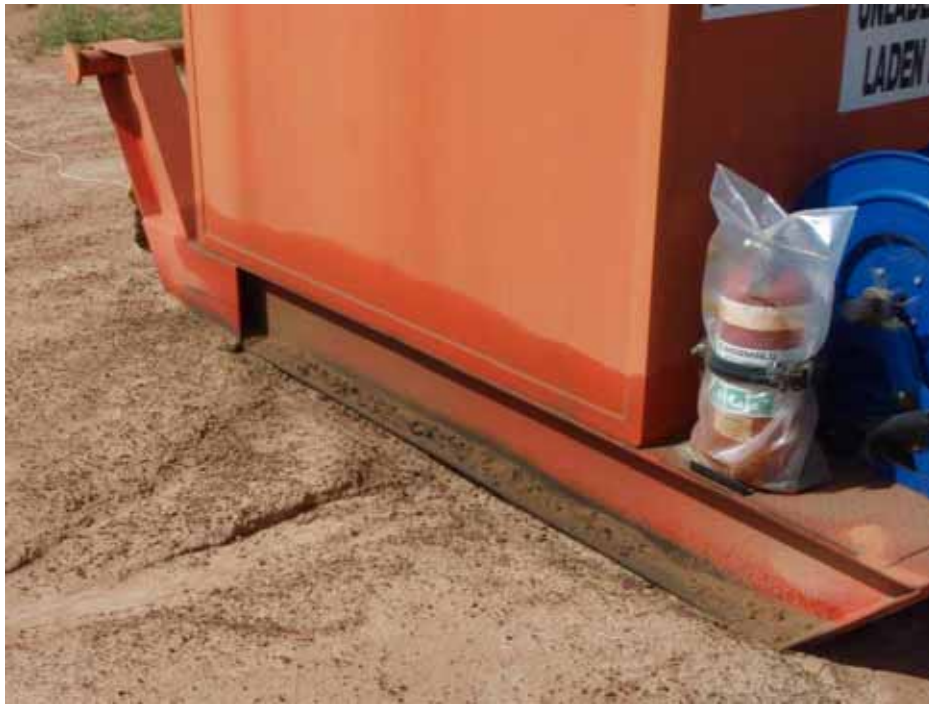
Plate 33 Staining on tank skids – Peak Downs Mine
