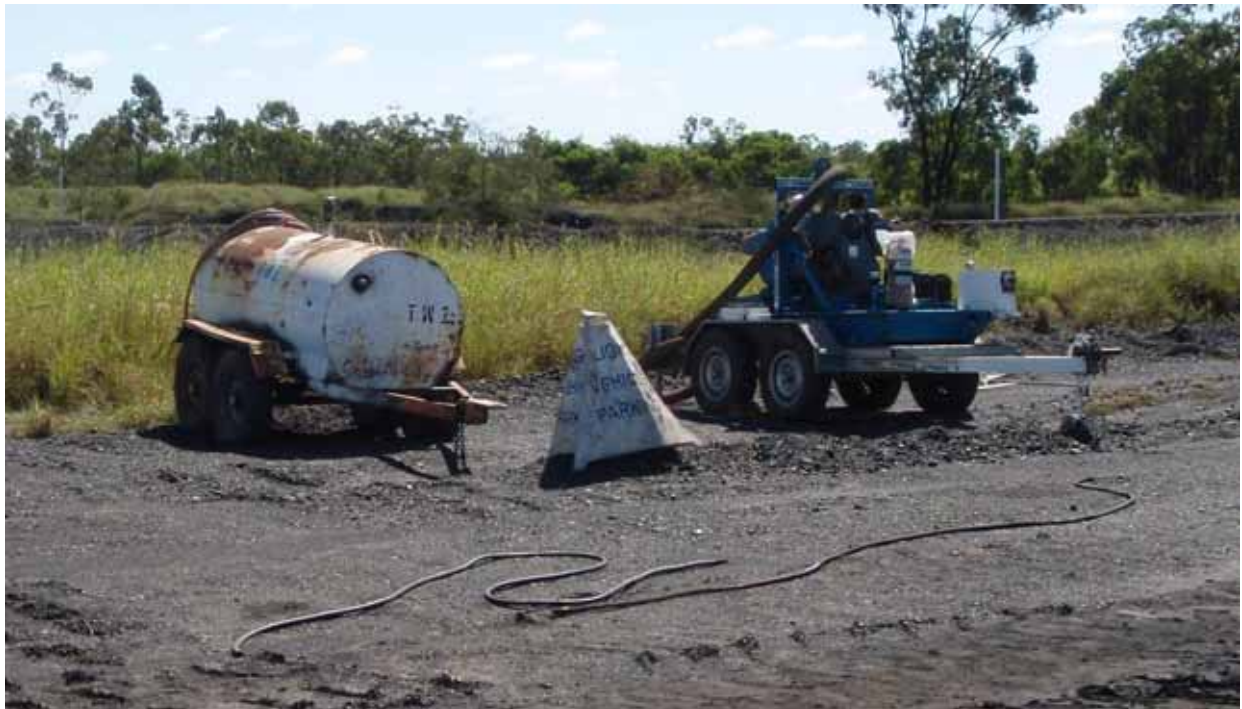
Plate 34 Mobile fuel tank and pump – Peak Downs Mine
