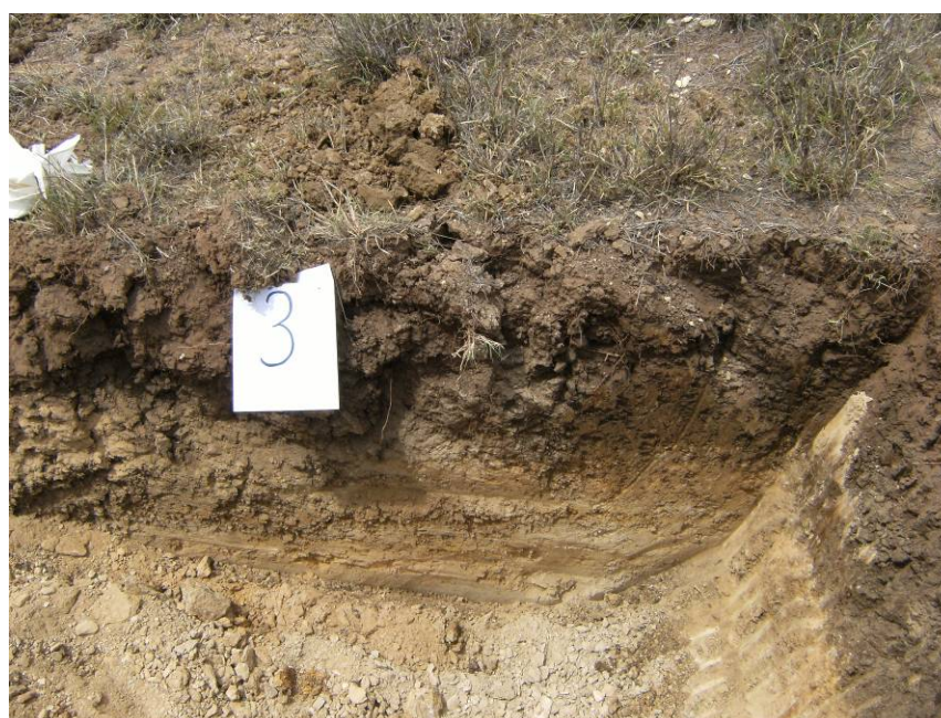
Plate 3 - Yellow Duplex Soil profile
