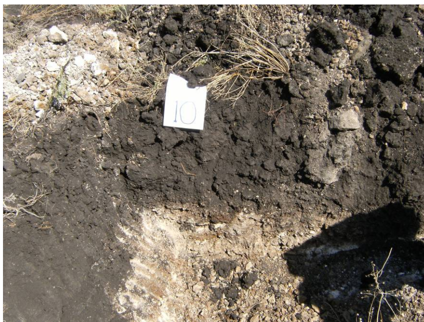
Plate 6 - Shallow Heavy Clay profile
