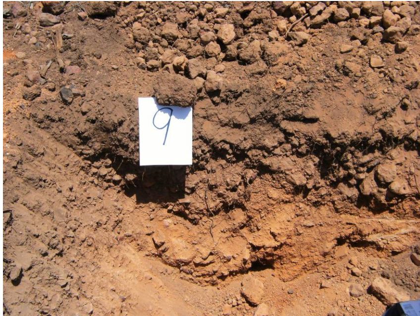
Plate 5 - Skeletal Soil profile
