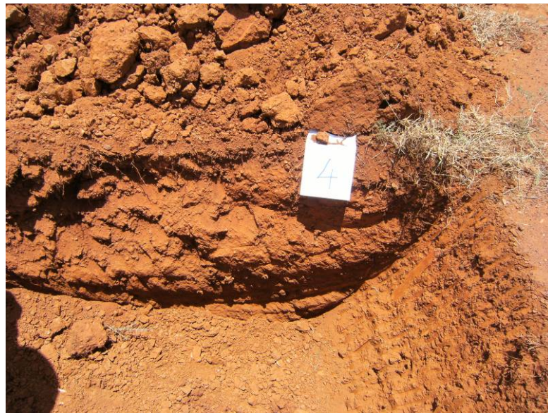
Plate 2 - Uniform Clay (red variant) profile
