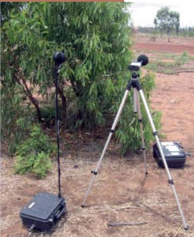
Noise monitoring equipment
