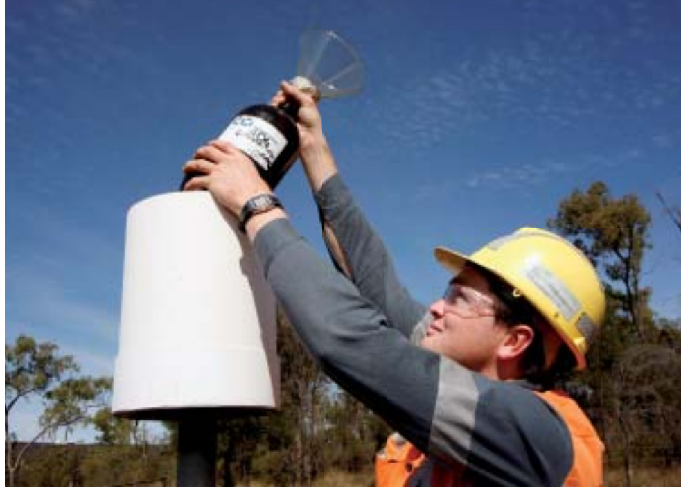
Figure 4 Example of dust deposition gauge installation
