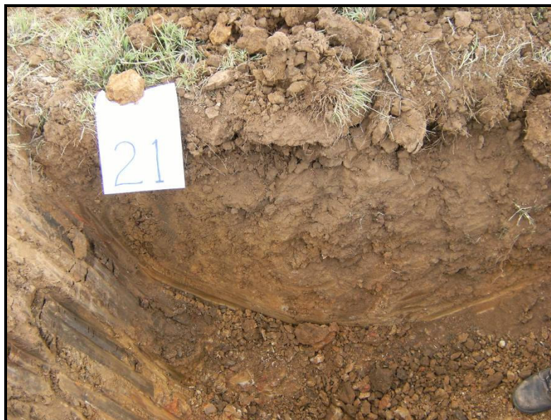
Figure 4.17 Uniform Clay Profile
