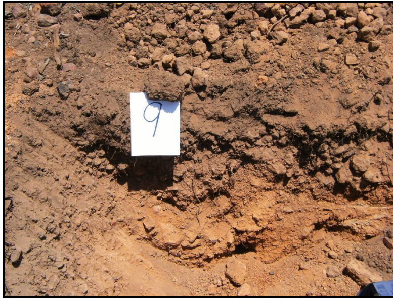
Figure 4.21 Skeletal Soil Profile
