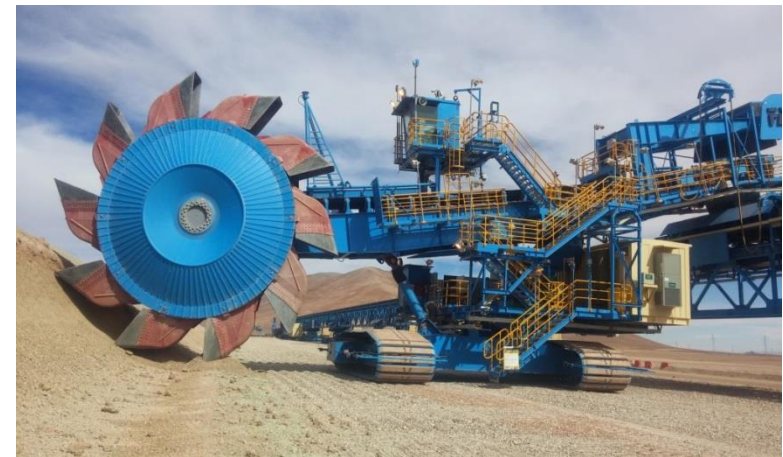
OLAP bucket wheel reclaimer
