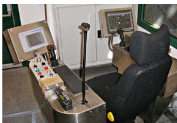
Operator's cabin from which the robot can be remotely controlled.
