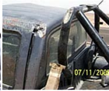
View of the external rollover bar showing no deformation
