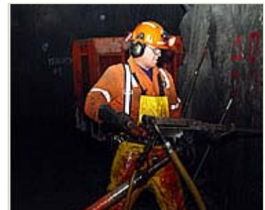
William Michelle, shown here training in the operation of a hand-held jackleg drill, is now an underground production driller
