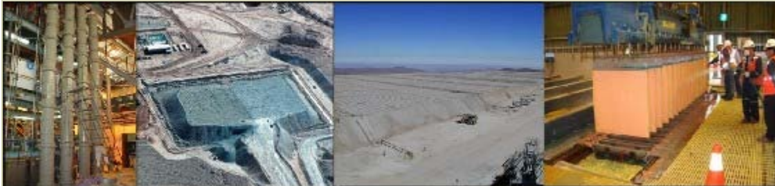
From left to right: Heap leaching R&D starts with studies in columns in a laboratory; may move to a demonstration scale heap; before full scale operation; all with the goal of producing copper metal.
