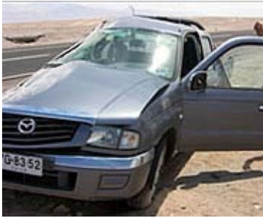
The vehicle overturned but there was no deformation of the interior and exterior rollover bars
