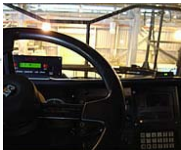
ASTiD technology that analyses driver/vehicle interactions to ascertain fatigue (e.g., steering corrections)
