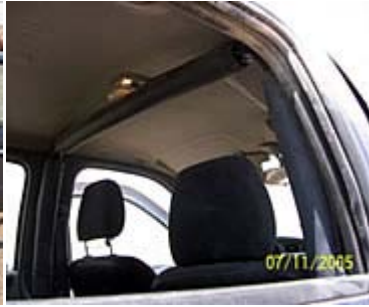
View of the interior rollover bar showing no deformation
