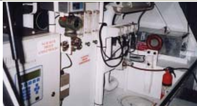
► Raw exhaust analyser at Elouera Colliery
