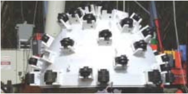
► Drill head used in blind bore rotary drilling
