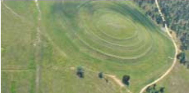
► Spiral contour drain at South Witbank
