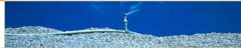
Right: A sprinkler is used to reticulate acid on top of the gold heap-leach stockpile at St Ives.
